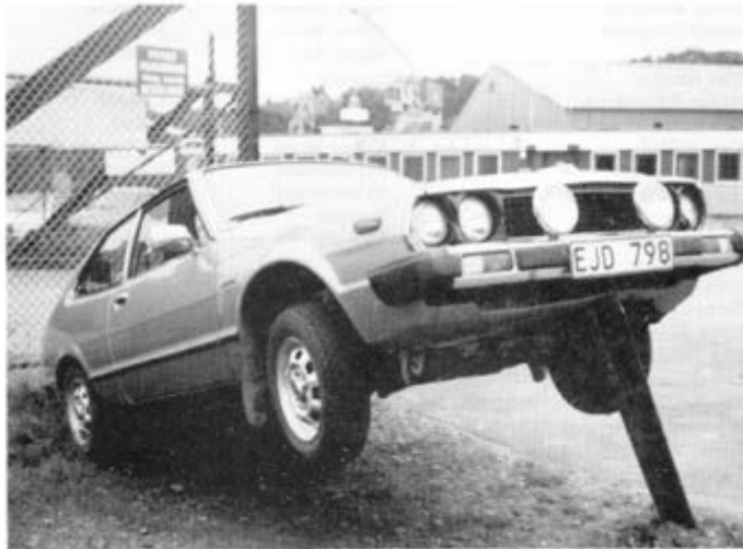
Fig. 1 The car with its front suspended by the pile hitting it from below
